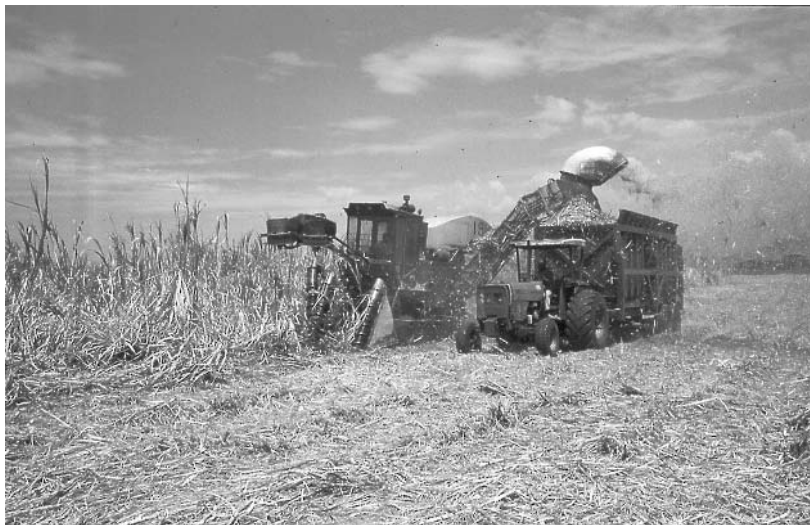
Fig. 9.7. Trash harvester replaced preharvest burning. About 10–20 Mg trash/ha remains after the harvest and the trash slowly decomposes.
