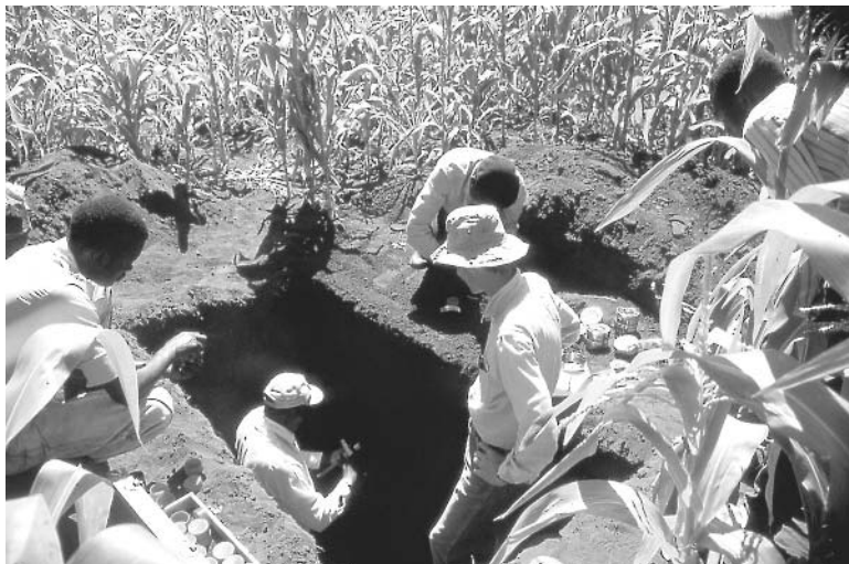
Fig. 4.7. Bulk density measurements in a Kandic Paleustalf soil pit of a maize field near Machakos (Kenya). Three 100-ml cores were used per horizon. Soil moisture content at the time of sampling is an important factor for correct measurements of the bulk density.
