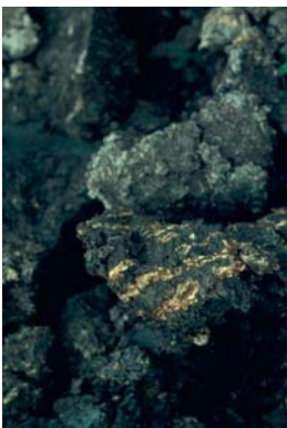
Electronmicrograph of pyrite in a sulphidic soil the result of bacterial reduction of sulphate in waterlogged conditions, the growing crystals also scavenge heavy metals and arsenic from the environment
